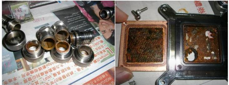
The purpose of experiment: Soak two different connectors in high metal ion coolant and Jingway low conductivity coolant, and after a period of time :
