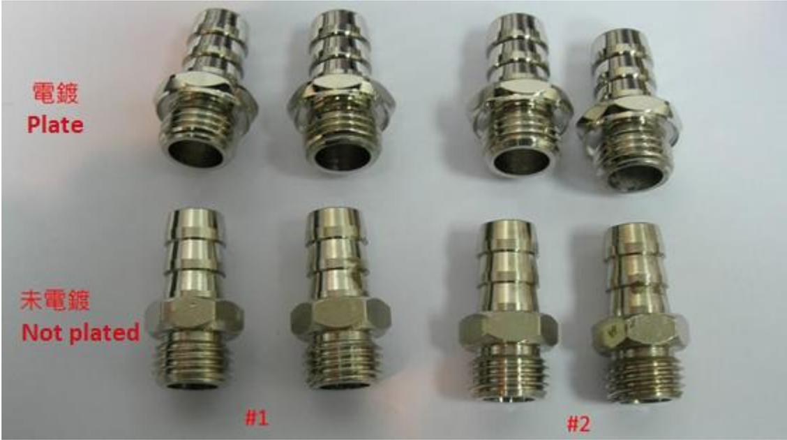
Figure 1- Before putting in the coolant 2009.12.16 (flaw means not plated)
